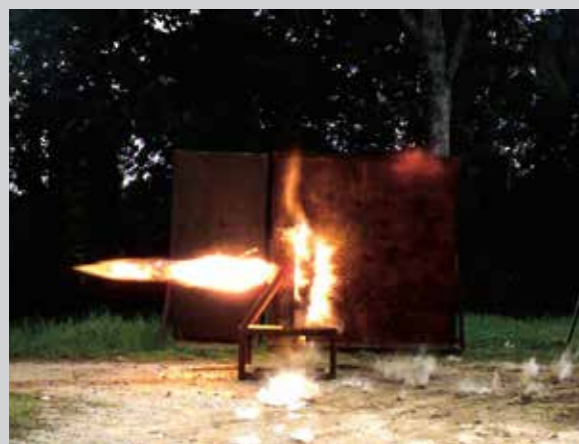
Penetration of 78mm RHA plate by HEDP cartridge
